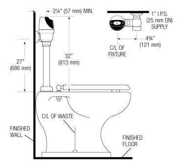
The Model 8116 valve is designed for installations where the water supply is roughed-in 27" (686 mm) above the top of the water closet.
